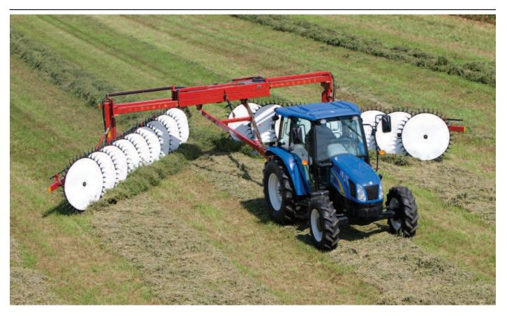
The NEW H5980 heavy-duty wheel rake is the perfect match for high-capacity hay growers. With eight 60-inch raking wheels on the left side and nine on the right, the H5980 rakes an area up to 30 feet, 3 inches wide. This offset design turns all of your crop, ensuring uniform crop drydown and eliminating the need for a center kicker wheel.
