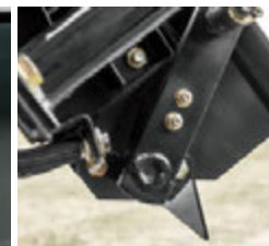
Stair position sensor.
