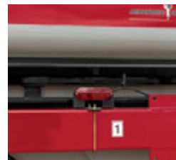
Tank full indicator lights.
