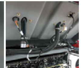
Tank pressure sensors.
