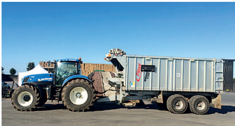
Fig. 4: New Holland T7 270 and Fliegl ASW 271 silage trailer combination with calibrated weighing system and trailer-side display
