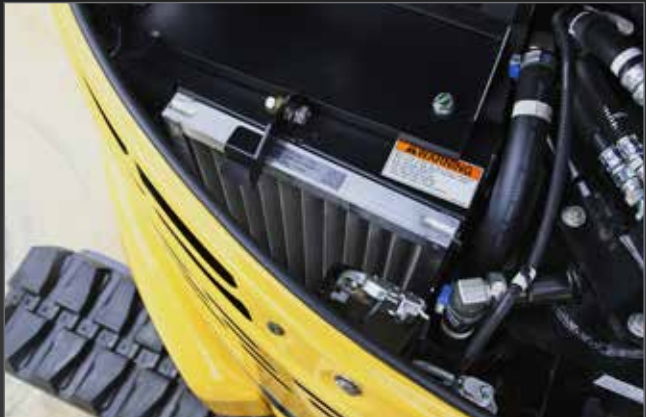
The iNDr filter has a high-density mesh of 30 lines per inch to collect dust.
