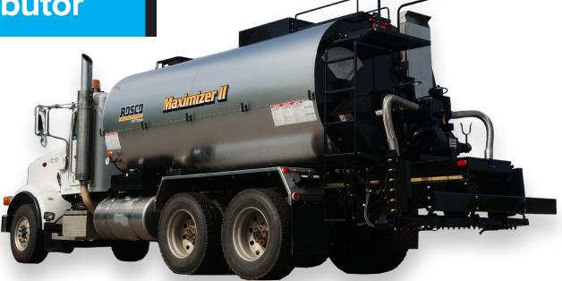
Applying a tack coat requires a sophisticated piece of equipment like the Maximizer 2B to ensure a uniform spray. The folding spray bar allows application without extensions and easily adjusts to provide even coverage of triple overlap fan spray pattern. Trusting in the proven reliability and solid performance that can only be found in a Viking asphalt pump coupled with our proprietary spraying algorithms, the Maximizer 2B yields long-lasting, top notch performance for all application types.
