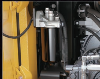
Engine Oil Filter Remote mounted for easy maintenance.
