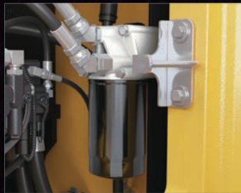
Fuel filters Main Filter / Pre-Filter with Integrated Water Separator.
