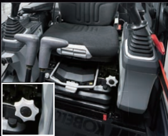
Adjustable Height Joystick Consoles The operator can adjust height of attachment control levers.
