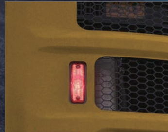
Swing Flashers for a Safer Jobsite Standard swing flashers notify ground workers that the machine is swinging.
