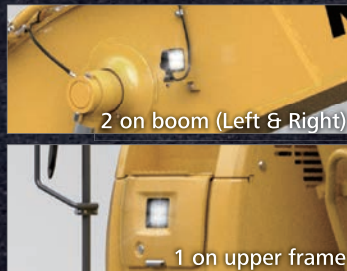
Standard 7 LED Lights Bright LED lights ensure visibility even during night work.
