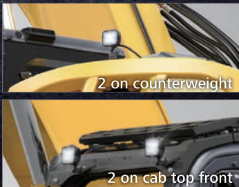
Swing Flashers for a Safer Jobsite Standard swing flashers notify ground workers that the machine is swinging.
