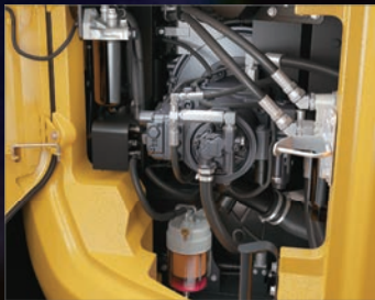
Right Side (Ground Level Maintenance) Hydraulic pump and engine filter compartment.
